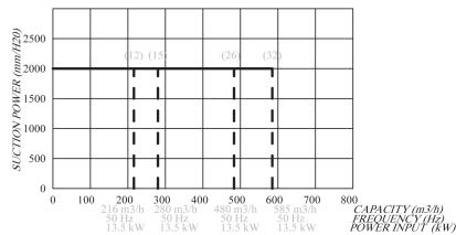
THE NUMBERS IN BRACKETS ARE WORKING PLACES THAT CAN BE SERVICED AT THE SAME TIME. - FIGURE CALCULATED USING AIR CONSUMPTION OF 18 m3/h  $\,$
