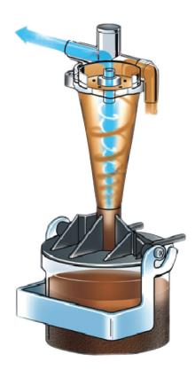
The liquid coming from the Turbo-Smart (as draining pump) rotates down the hydrocyclone and reverses direction and rotation when it reaches the narrowest section of the cone: at this point the particles of amalgam are deposited on the bottom of the tank connected to the hydrocyclone's cone while the liquid, cleaned of amalgam, exits at the top of the cone. The ISO hydrocyclone has a capacity of 18/l min.
